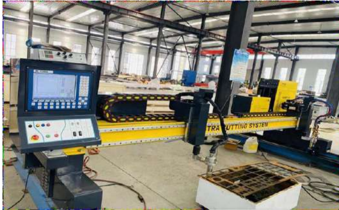
ASTRA MASTERCUT 200I Gantry CNC Cutting Machine. 1 Oxyfuel and 1 Plasma Station Working Table – 7000 mm x 3000 mm Up to 100 mm Thick
